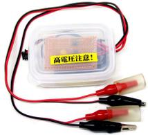
A Cockcroft high voltage unit supply up to 2kV tension. It sweep motley ions in air that achieve high efficiency and all weather operation.
