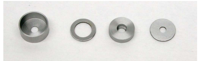
D3 Specimen holder manufactured in Japan using Mo-TEM alloy.
