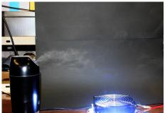
The droplet collection examinations were conducted in a clean bench with a wind speed of about 0.6 m/s. The number of large particles decreased with distance. This may be due to both falling by gravity and shrinking by evaporation. It was confirmed that the droplet removal system significantly reduced the number of droplets at the level of the face when a person seated at a table.
