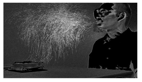
Special video recording was conducted to visualize droplets in the air. Within a range of about 50cm, we can see that droplets emitted by speech from the oral cavity with a "booming" sound are inhaled and stopped by the filter in the same way as a mask.
