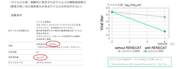
The amount of photocatalyst applied is about 0.7 g/m<sup>2</sup> in the standard specification of Hikari Cleaner, but it is about 14.3 g/m<sup>2</sup> in the high-performance filter that can be mass-produced. The illuminance on the filter surface of the Hikari cleaner is more than 68,500 lux. Therefore, the Hikari Cleaner is expected to inactivate at a faster rate than the above conditions.
