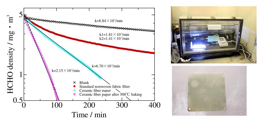
Using a 38L size acrylic desiccator, changes in the concentration of formaldehyde (HCHO), a kind of organic gas, were measured using a Formaldiameter htV-m.
