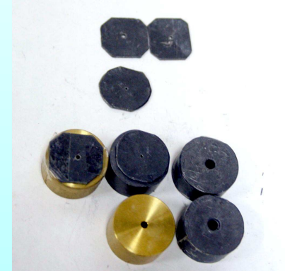
Collimators \phi 0.5 lead thin plate \phi 1.0 lead thin plate \phi 2 co-axial brass \phi 3 co-axial lead
