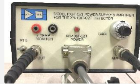
Power supply and Amplifier (PX2T, Amptek Inc., USA)
