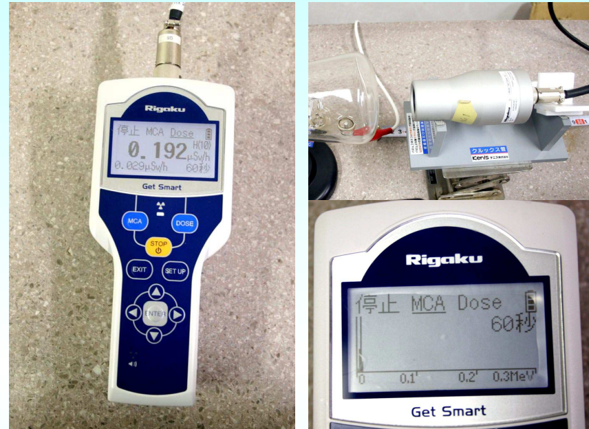
Rigaku Get Smart XU NaI scintillator Range 5 ~ 300keV (~10 \mu Sv/h)
