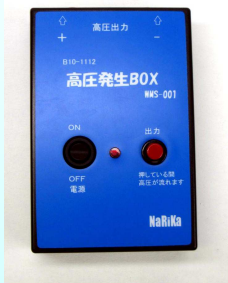
5kV CW high voltage unit driven by 9V battery
