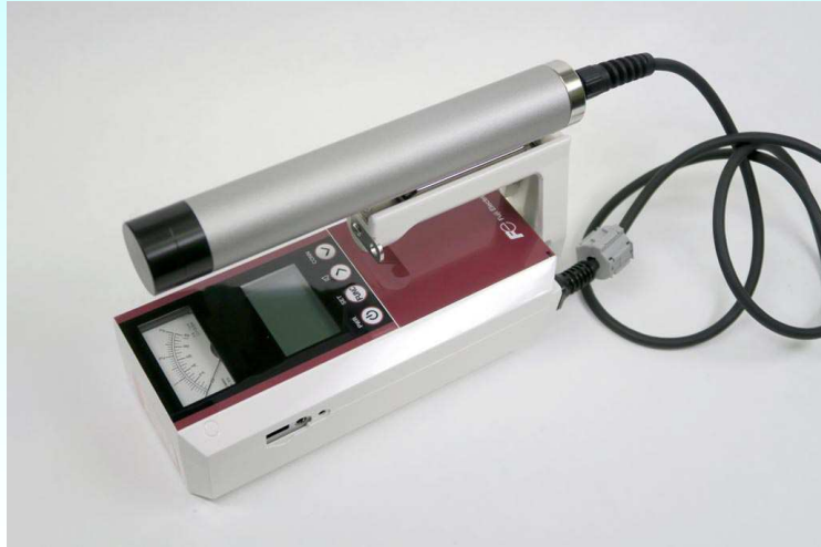
Fuji Electric NHC6 \phi 12.7 × 12.7mm NaI scintillator Range X-ray 8 ~ 300keV (~60 \mu Sv/h), \gamma -ray 50 ~ 1500keV (~600 \mu Sv/h)
