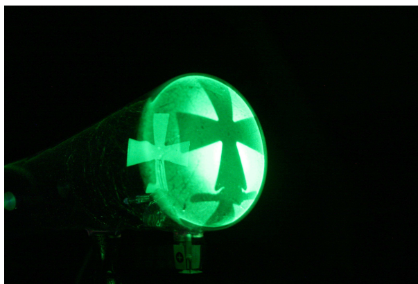
Fig.1 A Crookes tube in operation with a Maltese cross plate
